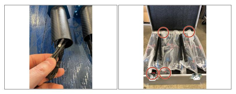
• Check the base of each arm to ensure that the motor wires get tucked into the carbon fiber arm tube. This will ensure that the motor wires do not get closed in the lid of the travel case.
