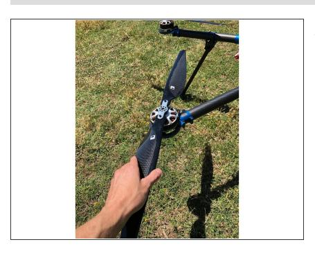
Ensure propellers are safe for flight (properly mounted and unfolded)
